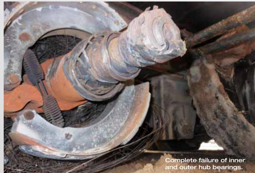
Complete failure of inner and outer hub bearings.
