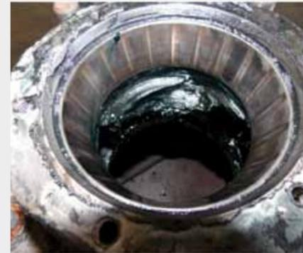
Wheel vibrations have produced characteristic wear marks on this mid-life bearing cup.
