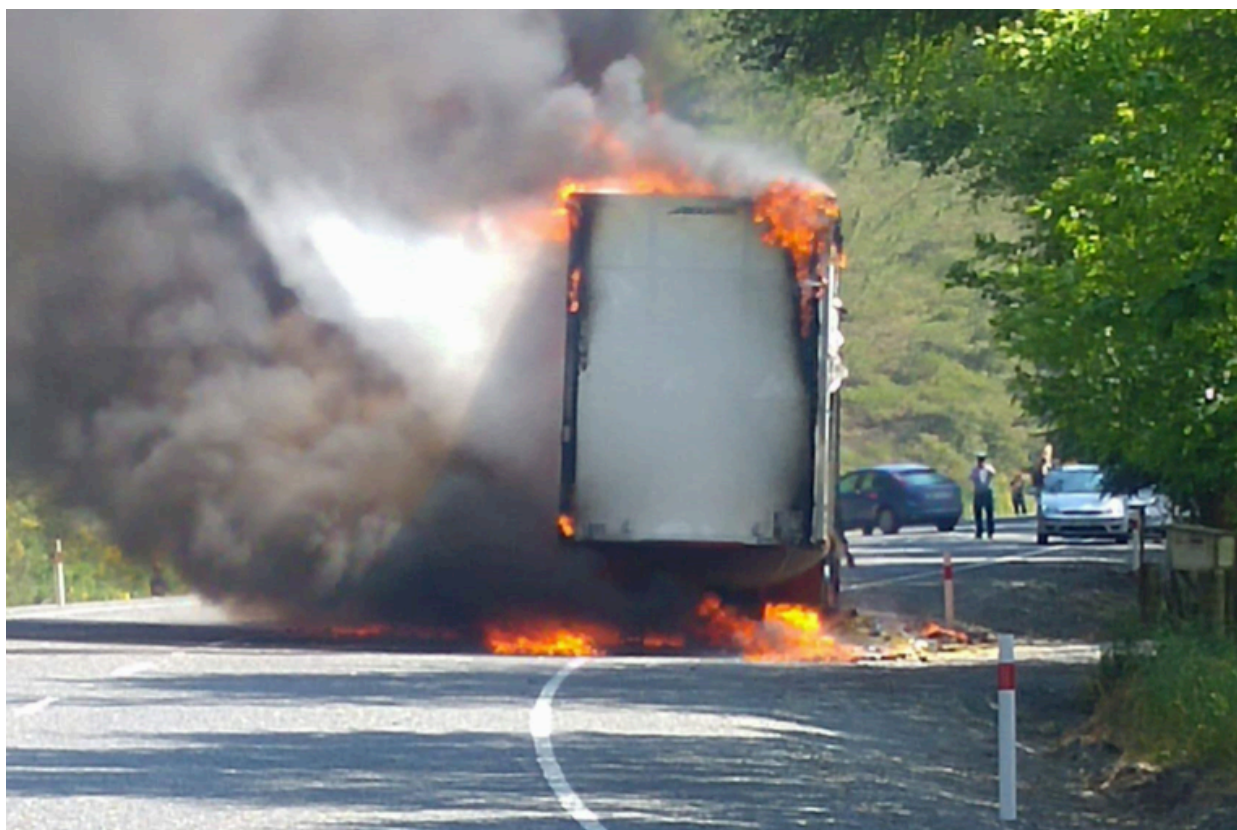
Figure 3: Photo of a trailer fire at early stages. Note the wind direction can be clearly identified. Taken by the driver.
