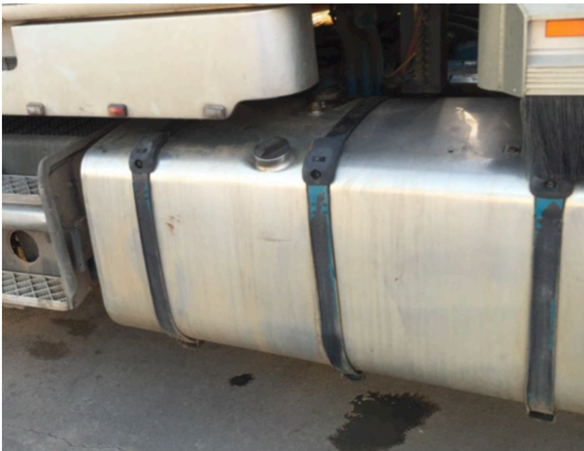
Figure 1: Driver observed a leak under the left-hand fuel tank at his next stop. But continued driving. The truck eventually caught fire.
