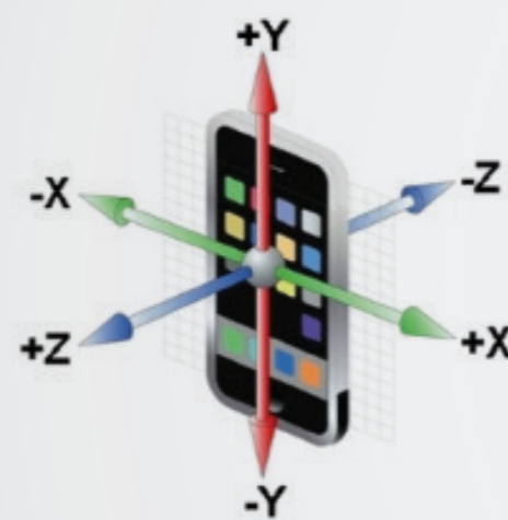
The mobile phone can measure vibrations in three directions.
