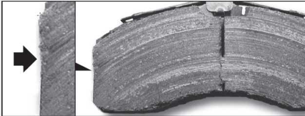
Brake Pad with minor damage (permitted)
