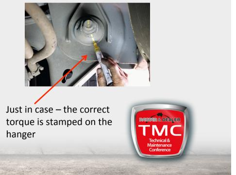
3. Checking the shock absorber orientation and shock bolts torque
