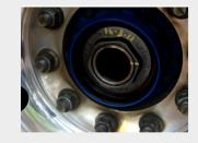
Left hand side – LH thread Right hand side – RH thread Torque: 900Nm
