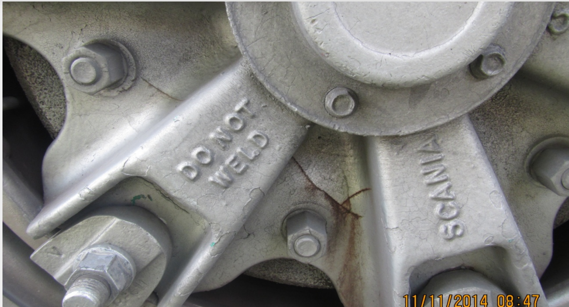
3 axle Scania carrying timber LHF spider hub cracked
