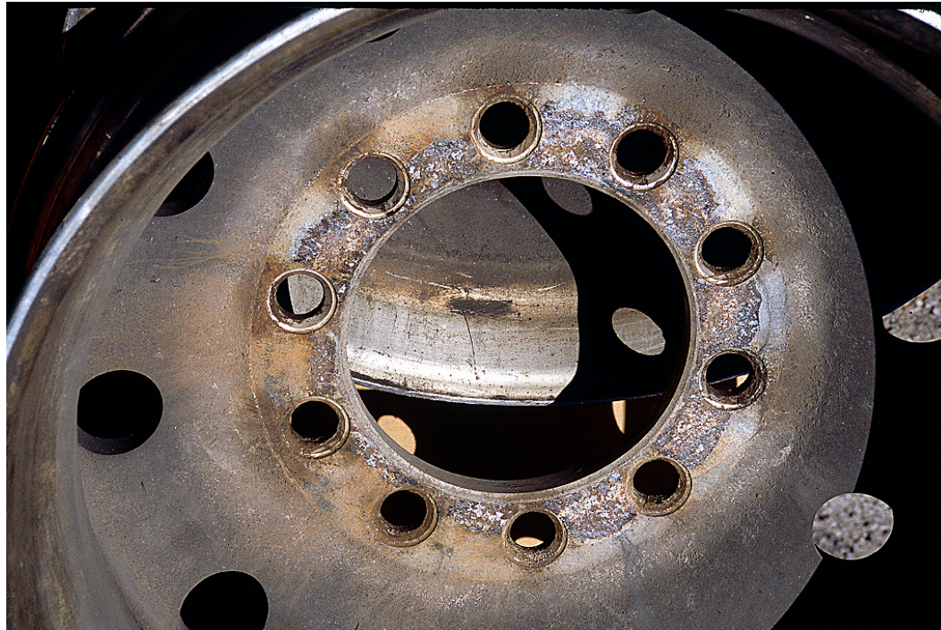
■ Mounting Surface Corrosion
