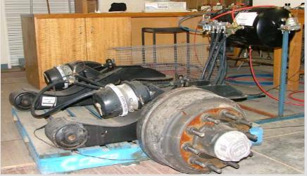
Overall system is connected with the maximum possible length of signal and air lines that will allow the system to meet the ADR.
