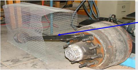
Meter long steel flat is attached to the brake drum with weights attached at the end. This will be used to determine the brake threshold pressure.
