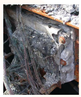
Aluminium can melt during a truck fire. Steel and copper do not, other than at arc points.
