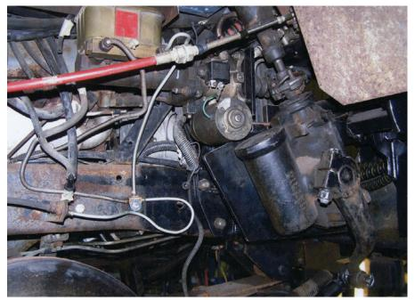
Failure of a brake hose in close proximity to the exhaust extractor pipes probably caused this fire.
