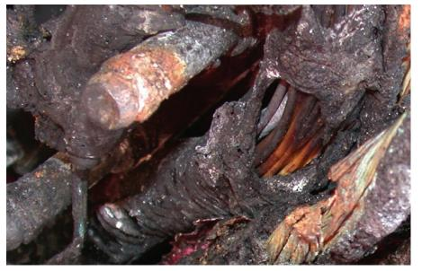
The result of a rub between the alternator cable and an engine stud. The alternator cable was double-insulated with a split-conduit covering but the split worked its way around to the stud position. It had no circuit breaker protection at the battery end.
