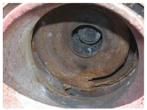
A failed turbo charger blade led to bearing failure and then seal failure. Oil pumped into the exhaust caused an exhaust-fire that destroyed the truck.
