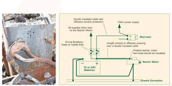
Above left: A starter motor cable tucked between a bolt stud and the battery box cover ignited this fire. The plastic conduit on the cable was split and the split worked around to the stud position. Note that the steel stud melted.
