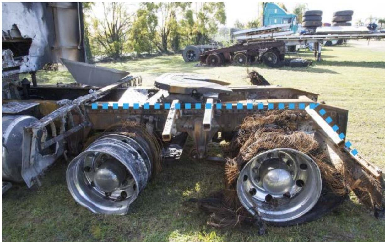
Bracket failures on heavy-duty mudguards.
