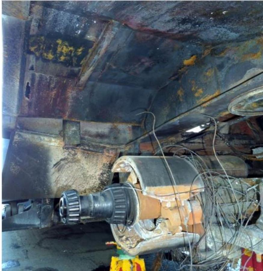
The air suspension deflated en-route and the tyres rubbed on the steel mudguard.
