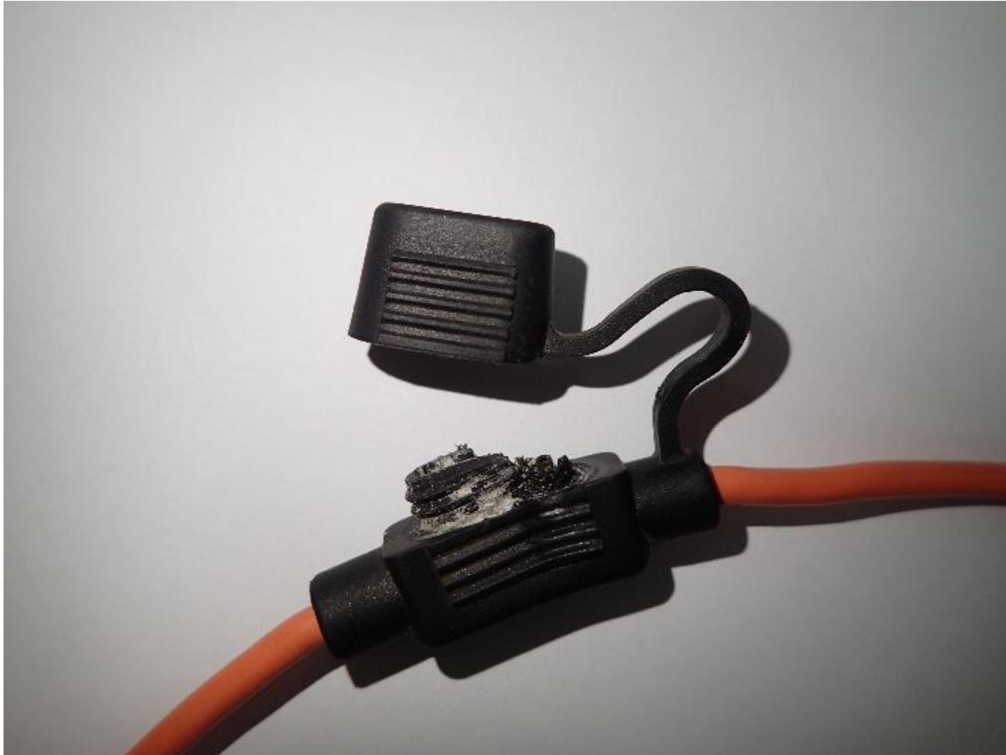
Carbonate filler comes out of the rubber when it gets hot.
