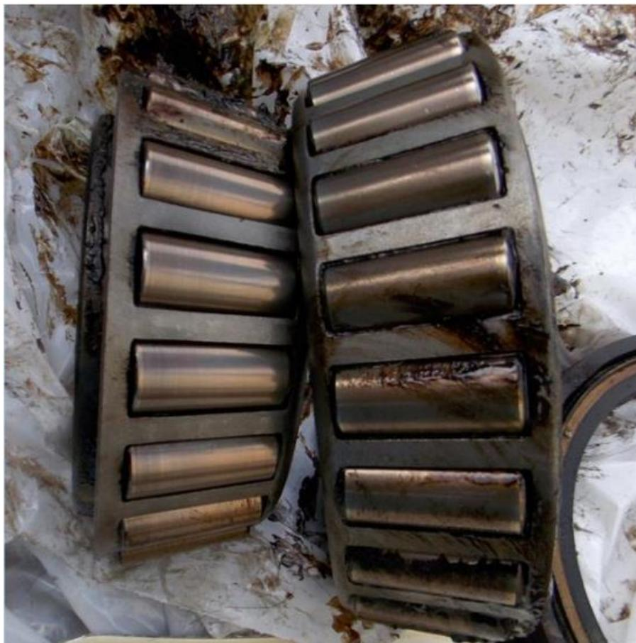
Distressed lubrication on new bearings from axle 2.
