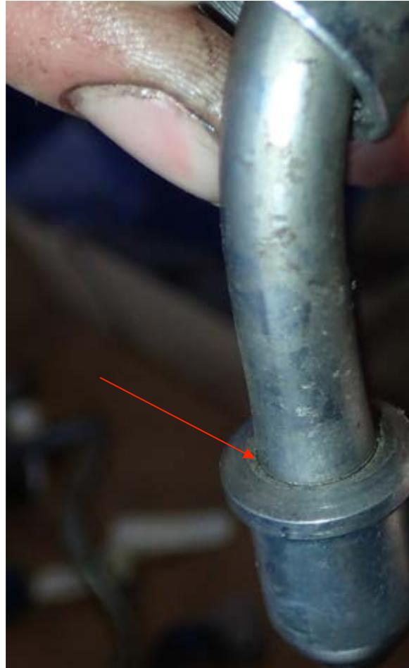
High pressure engine tube cracks.
