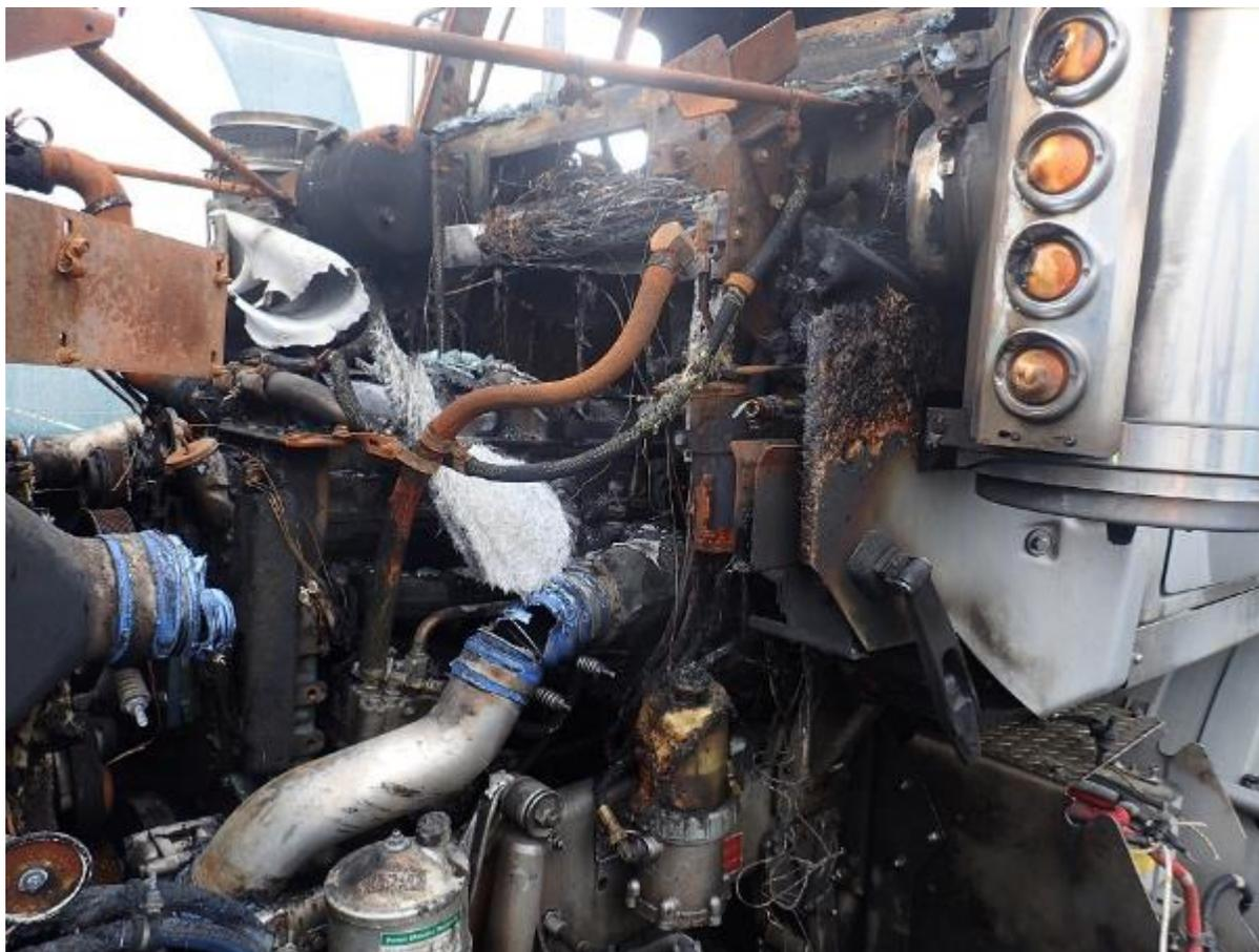
The fire appears to have started in the electrical compartment on the firewall underneath the windscreen.
