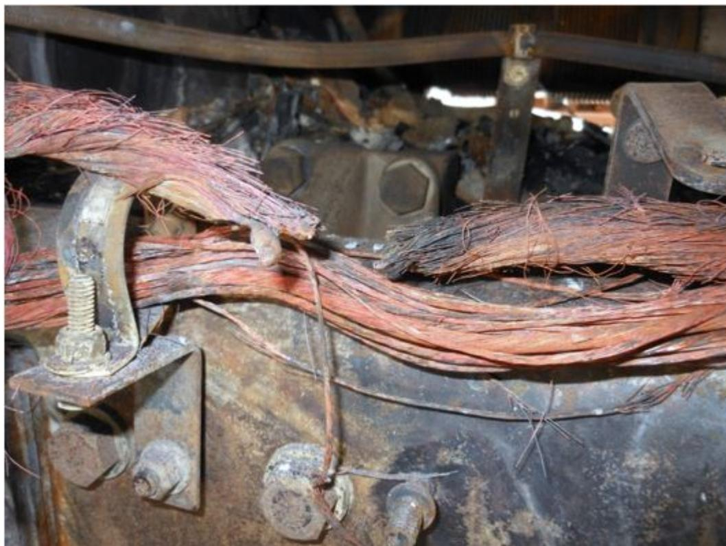
A rub on the positive battery cable at a steel-spined clamp point underneath the cabin.
