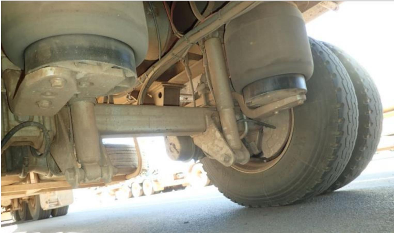
Air suspensions will deflate if a supply tube fails.
