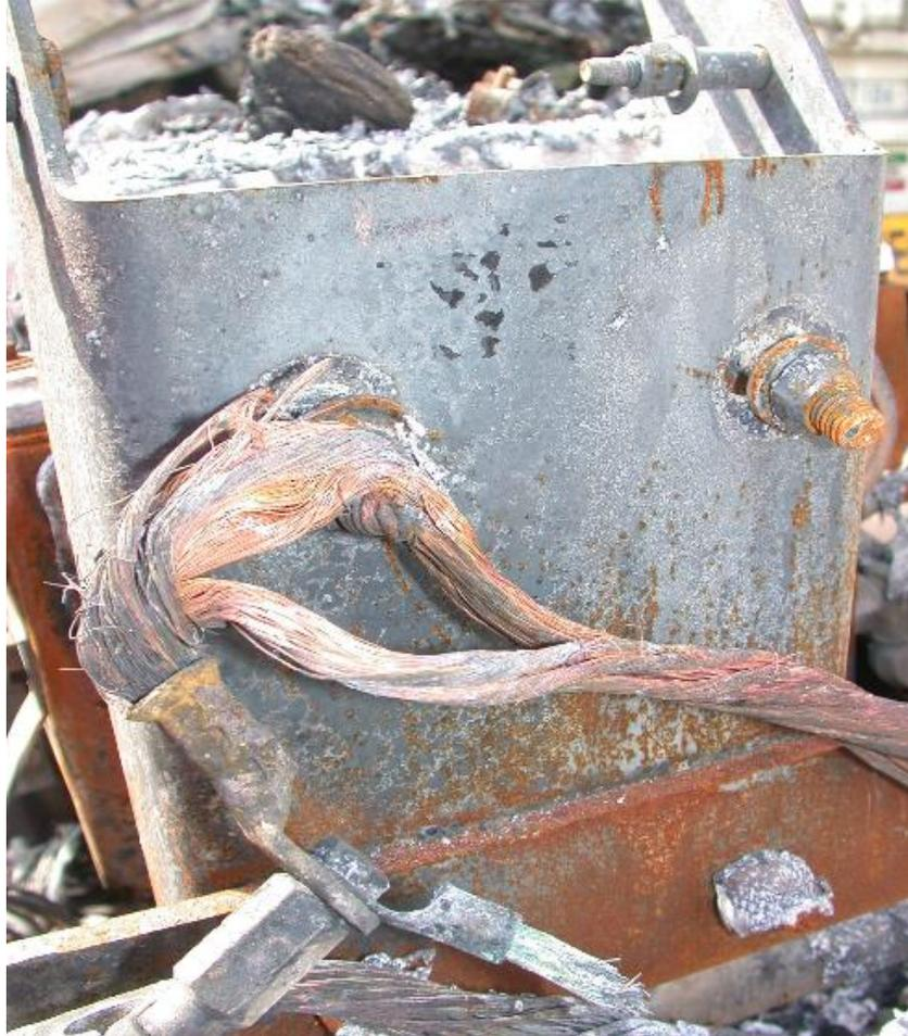
Rasping of the conduit and plastic led to a short-circuit.
