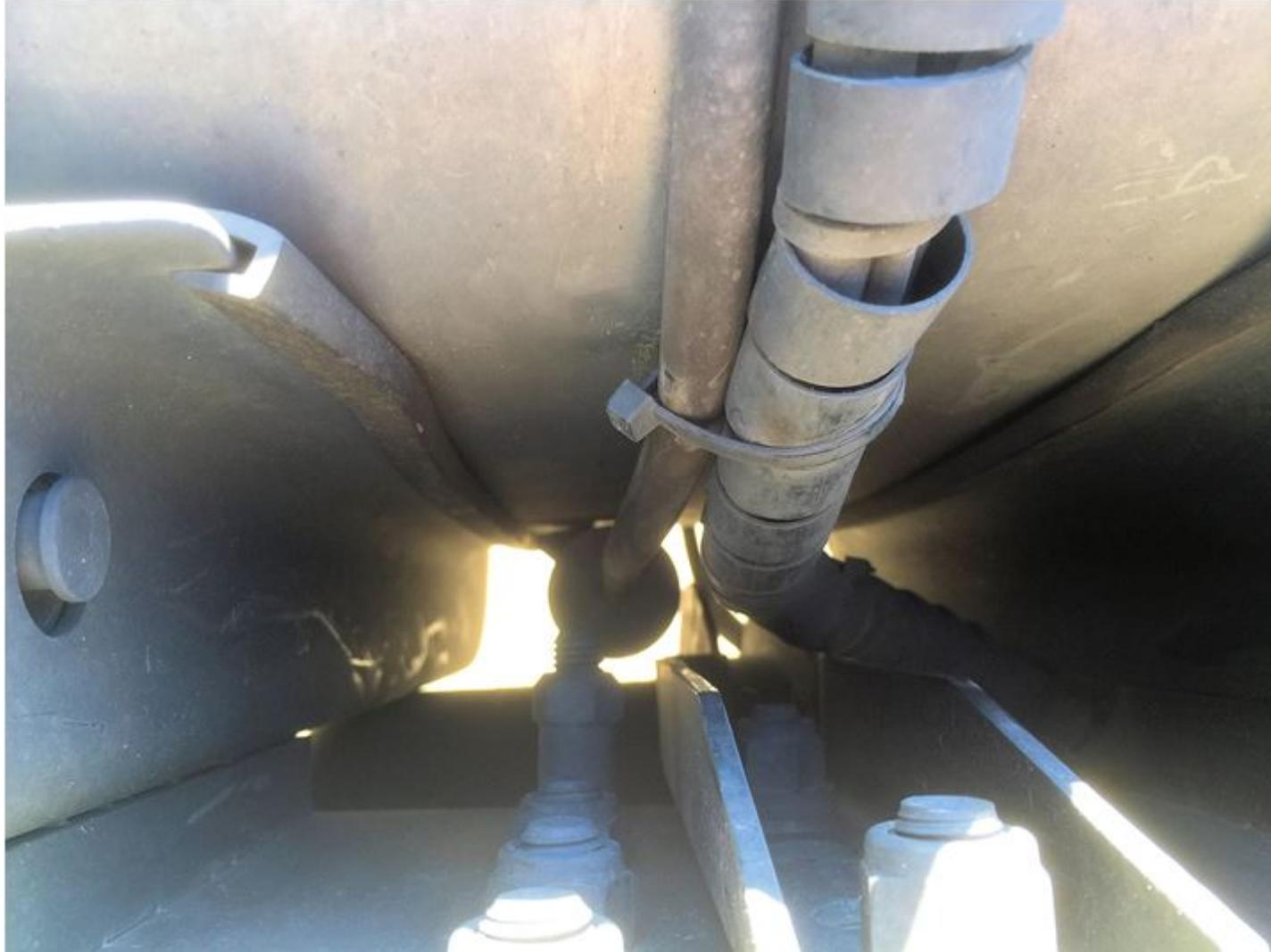
The fuel lines run down the side of the fuel tank.
