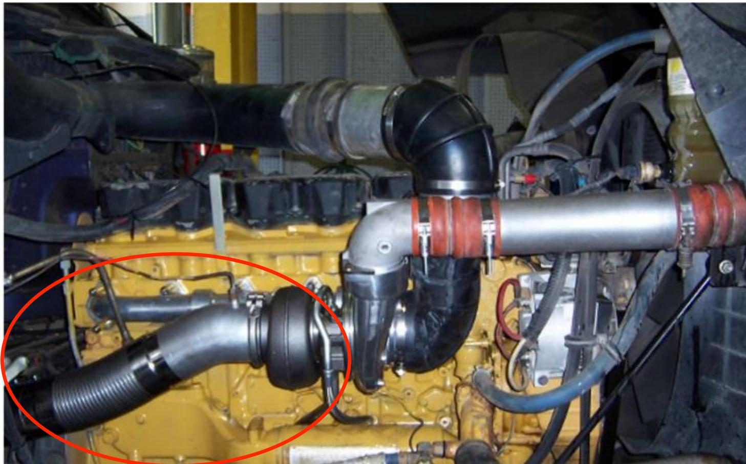
Only the exhaust and turbocharger are hot enough to ignite oil or diesel fuel.
