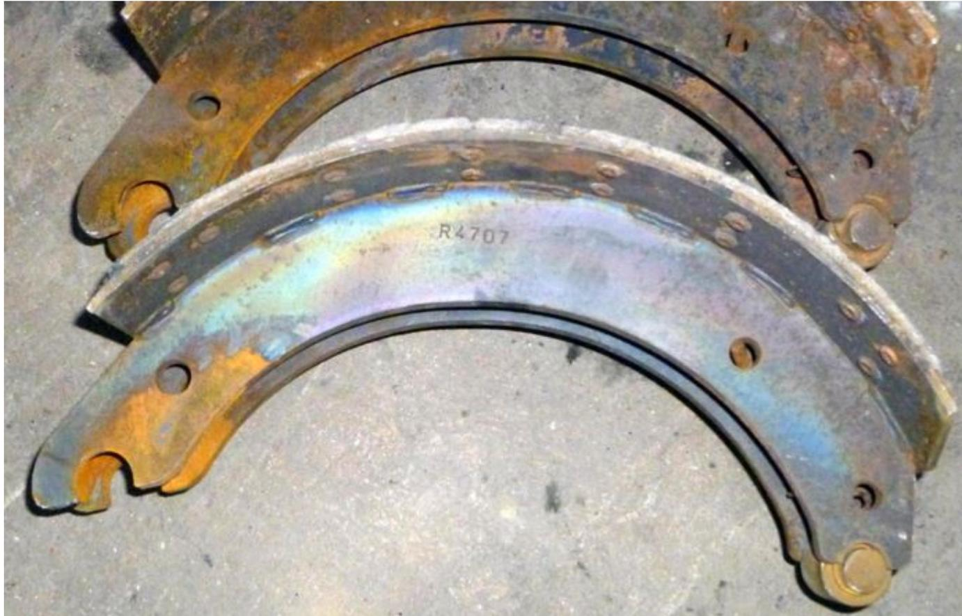
Dragging brakes cause extreme brake drum temperature.
