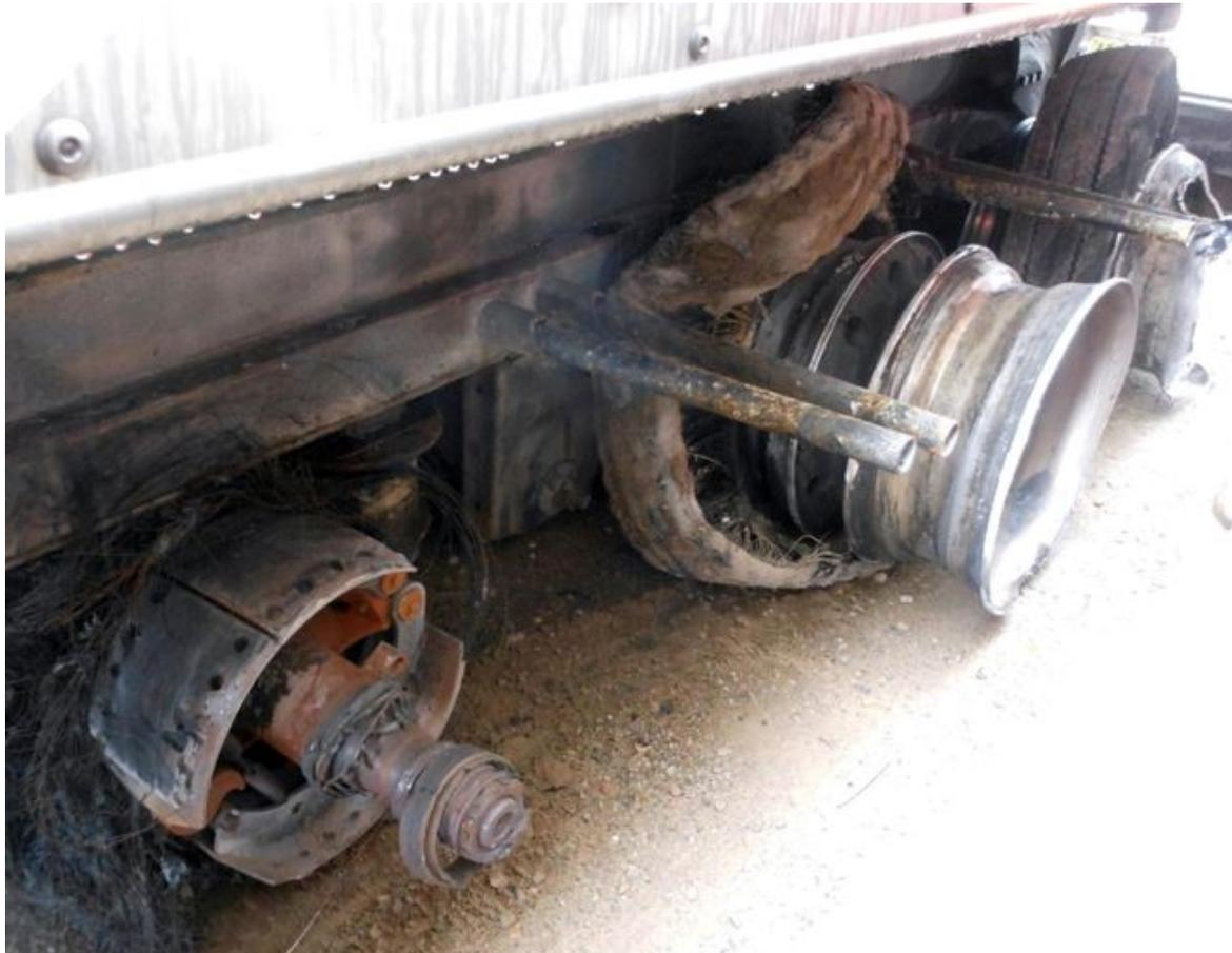
Mechanical failure of the bearings on the front axle is evident.
